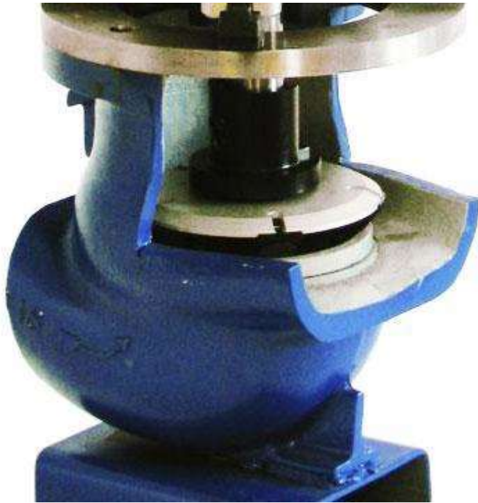
Model C - A portable, easy to mount, cutting, milling and grinding machine. Ideal for globe, safety and control valves
